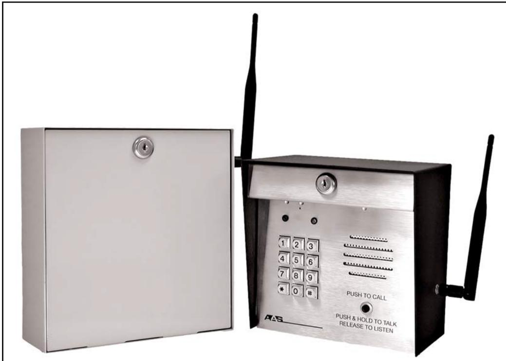
The American Access Systems **PhoneAire** is a fully digital, wireless telephone entry system. The transmitter is constructed using a heavy gauge, powder coated enclosure and stainless steel faceplate that mounts directly to a pedestal or can be surface mounted. The **PhoneAire's** receiver is mounted in a standard rain-tight enclosure with a baked enamel finish and mounts directly to the side of the home or main building. 2000 foot "Line of Sight" between gate unit and the receiver unit.
